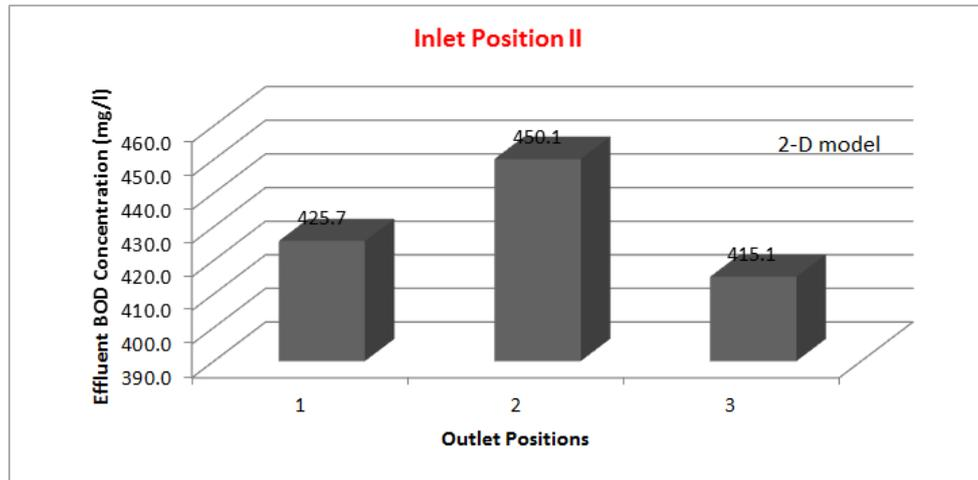
**Fig-7: Effect of single inlet/outlet position on WSP performance**
