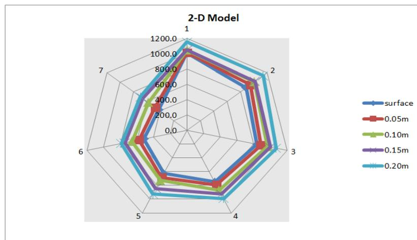
Fig-6: Variation of BOD Concentration with depth of pond
