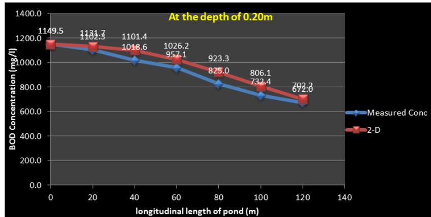
Fig-4: Comparison between measured value and CFD model using inlet position I
