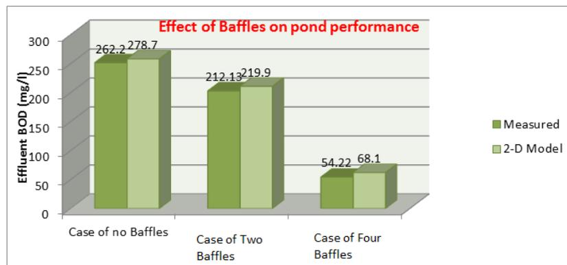
Fig-5: Effect of baffles on pond performance
