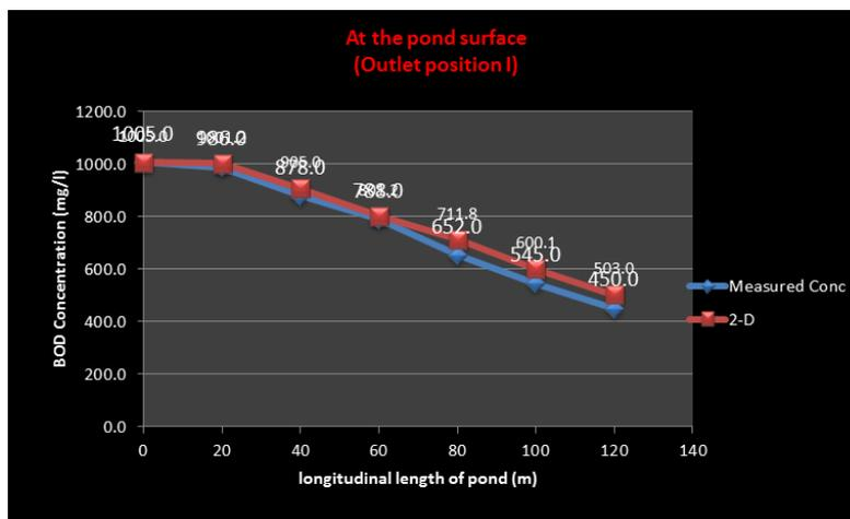
Fig-2: Comparison between measured value and CFD model using inlet position I
