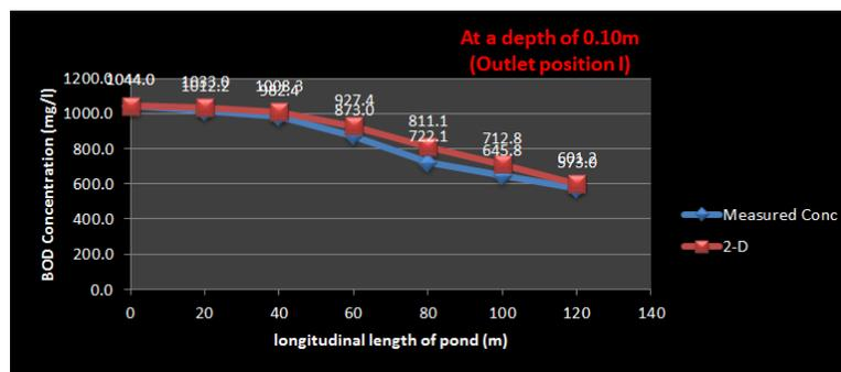
Fig-3: Comparison between measured value and CFD model using inlet position I
