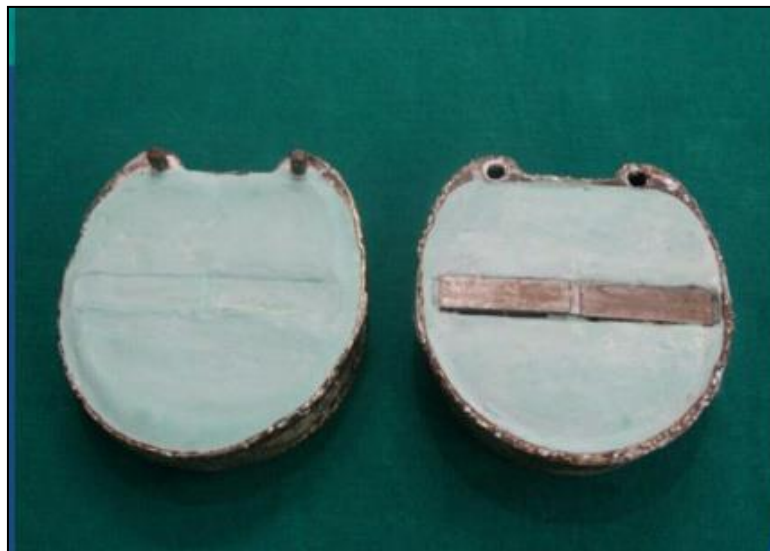
Fig. 2: Metal die invested in a flask
