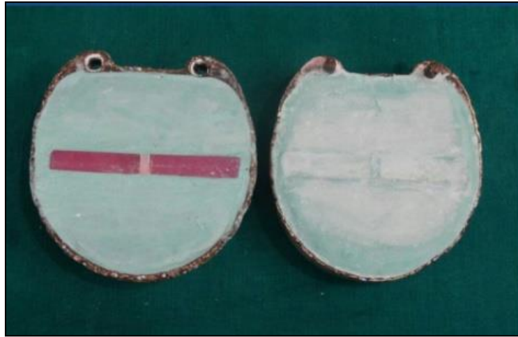
Fig. 3: Metal die replaced with two polymerized acrylic block with silicone soft liner in between cure acrylic resin and silicone soft liner in between
