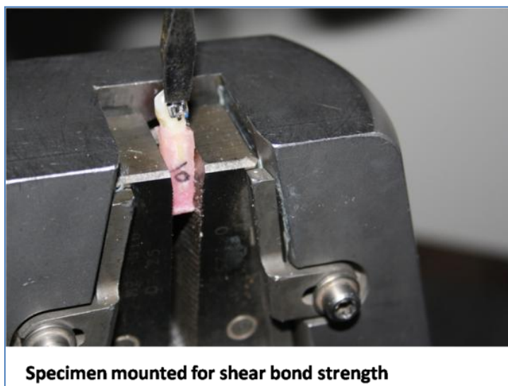
Fig-4: Mounted Specimen for checking Shear Bond Strength
