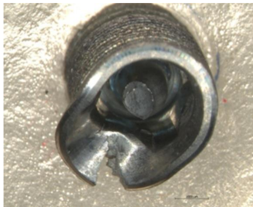
Figure 3: Fixture and screw fracture failure mode revealed by Stereomicroscope (magnification 1000 \mu\text{m} ), (top view).
