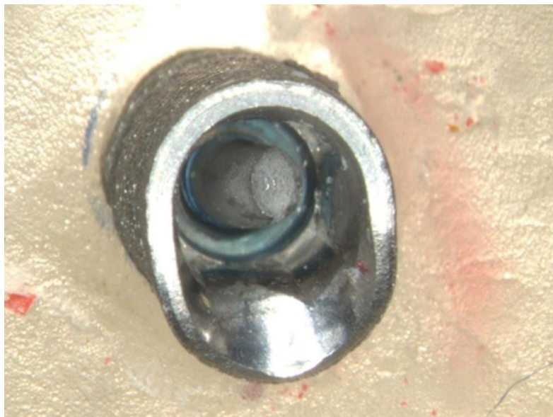
Figure 5: Screw fracture failure mode with fixture neck deformation revealed by Stereomicroscope (magnification 1000 \mu\text{m} ), (top view).
