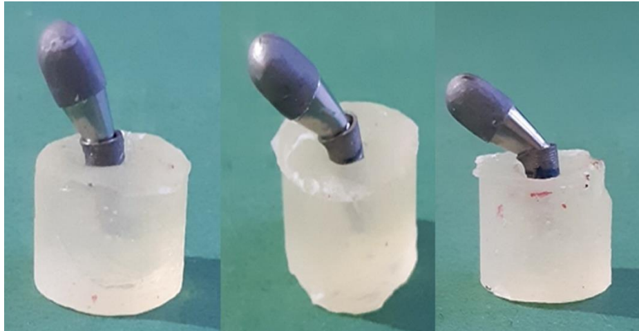
Figure 1: Deformation of dental implant specimens.
