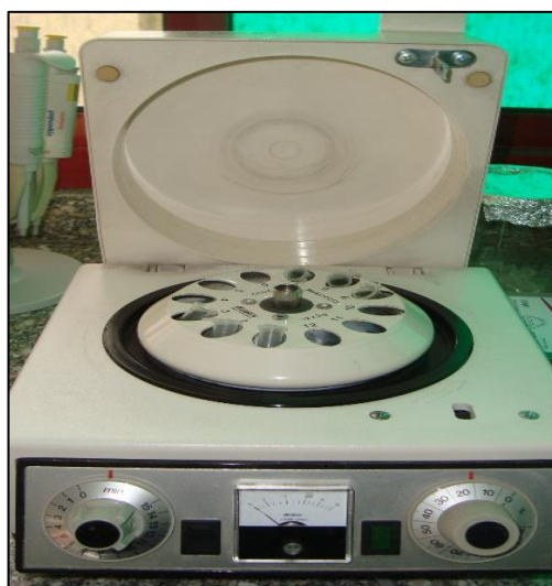
Figure 1: Samples were centrifuged at 4000 rpm for 20 minutes
