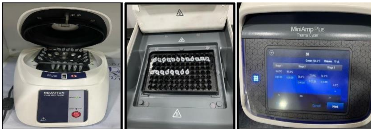
Fig. 7: Polymerase chain reaction by thermal cycler
