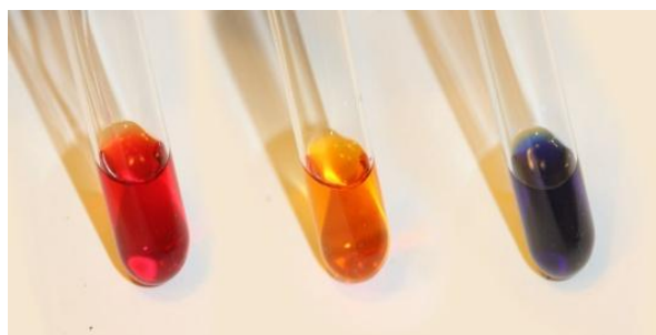
Fig-1: Color change of Thymol blue in acid (red) and alkaline (blue) medium.
