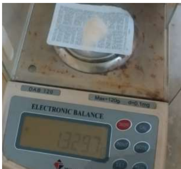
Fig. 3: Measuring the desired weight of NaNO 3 by using weighing Machine
