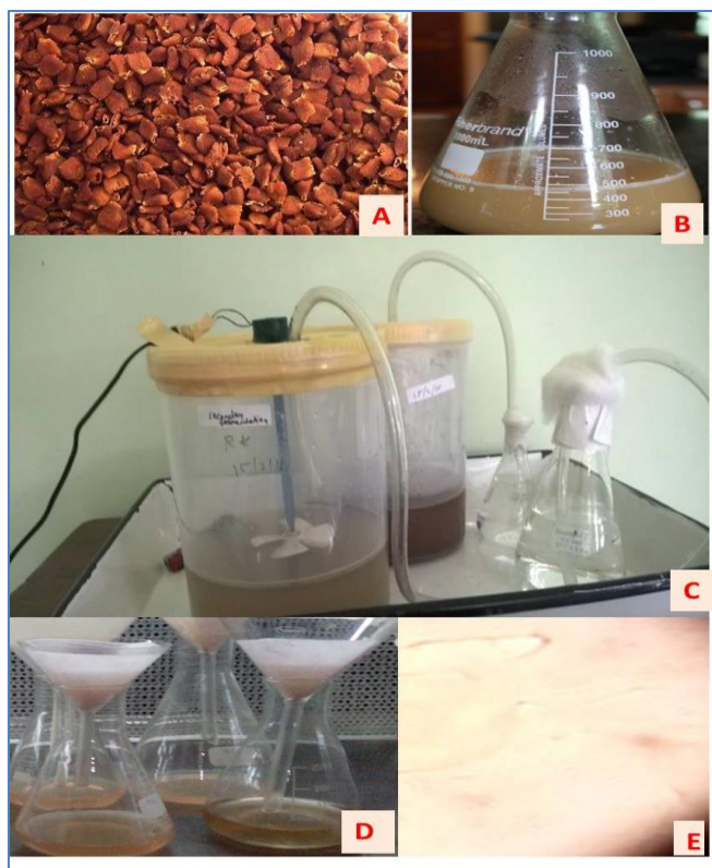
Fig-2: A-E showing different steps of production of wine. Dry flower of Mahua (A); Yeast inoculant (B), Fermentation apparatus (C); Microscopic photo graph showing no traces of yeast in the sample (D) Filtration of the sample through filter paper (E).
