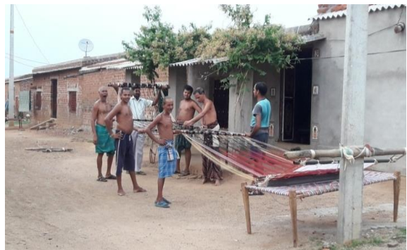
(Weavers folding the warp yarns after the end of the street sizing process)
