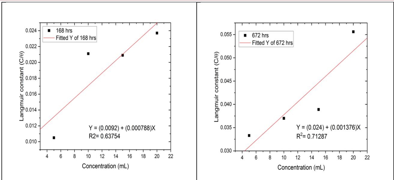
**Fig 11: The Langmuir adsorption isotherms for *Cnidoscopus aconitifolius* in 0.5 M NaCl solution at 168 and 672 hours exposure times**
