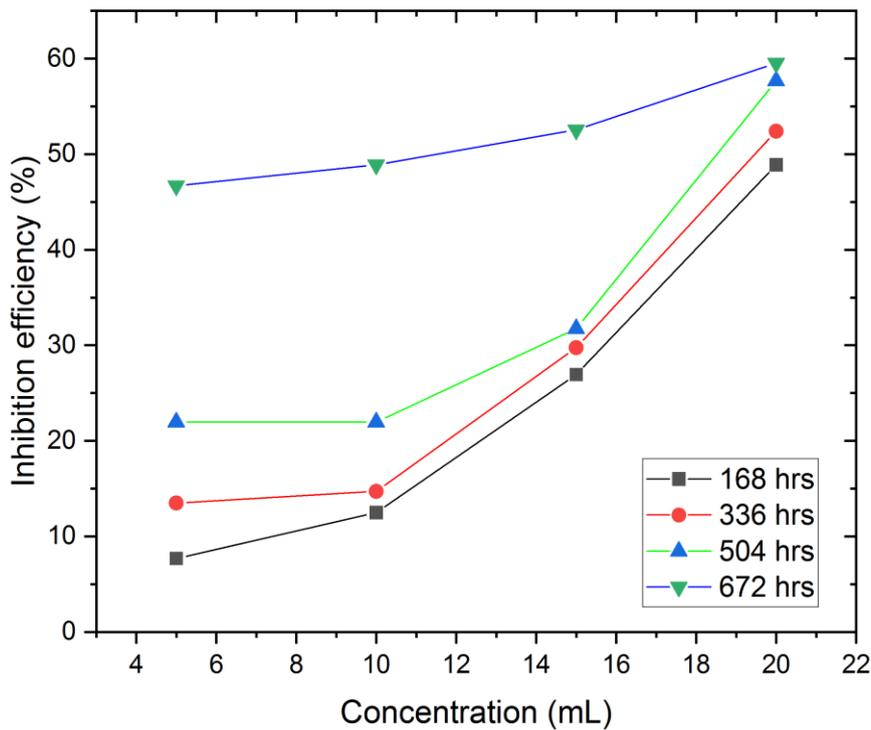
Fig 5: Inhibition efficiency against extract concentration for *Cnidoscolus aconitifolius* in 0.5 M H<sub>2</sub>SO<sub>4</sub>
