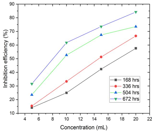
Fig 8: Inhibition efficiency against extract concentration for *Cnidoscopus aconitifolius* in 1.0 M NaCl solution
