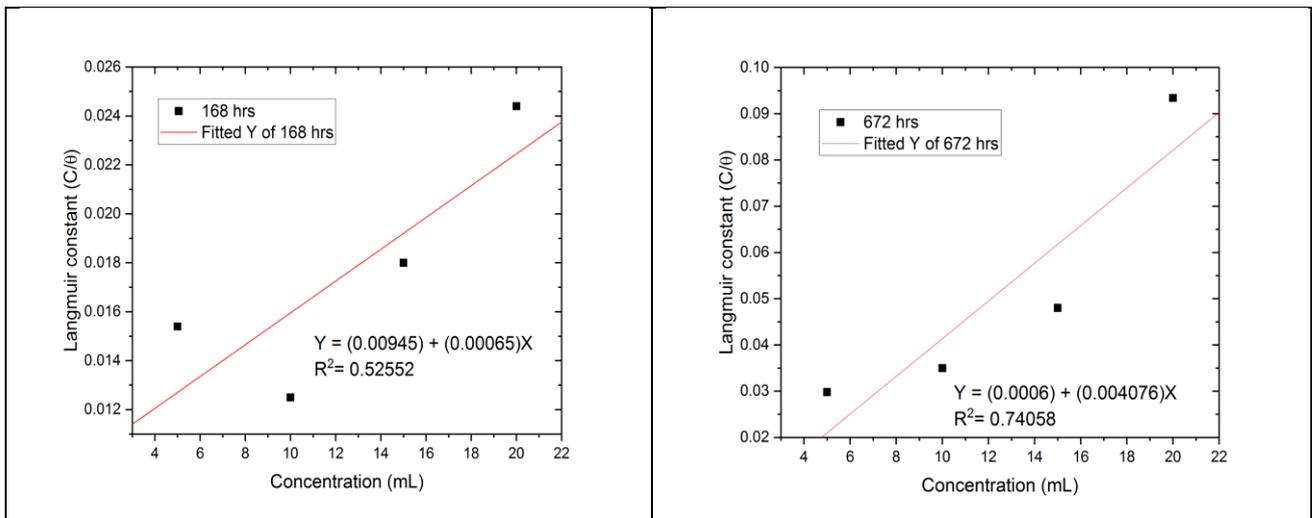
Fig 9: The Langmuir adsorption isotherms for *Cnidoscopus aconitifolius* in 0.5 M H<sub>2</sub>SO<sub>4</sub> at 168 and 672 hours exposure times
