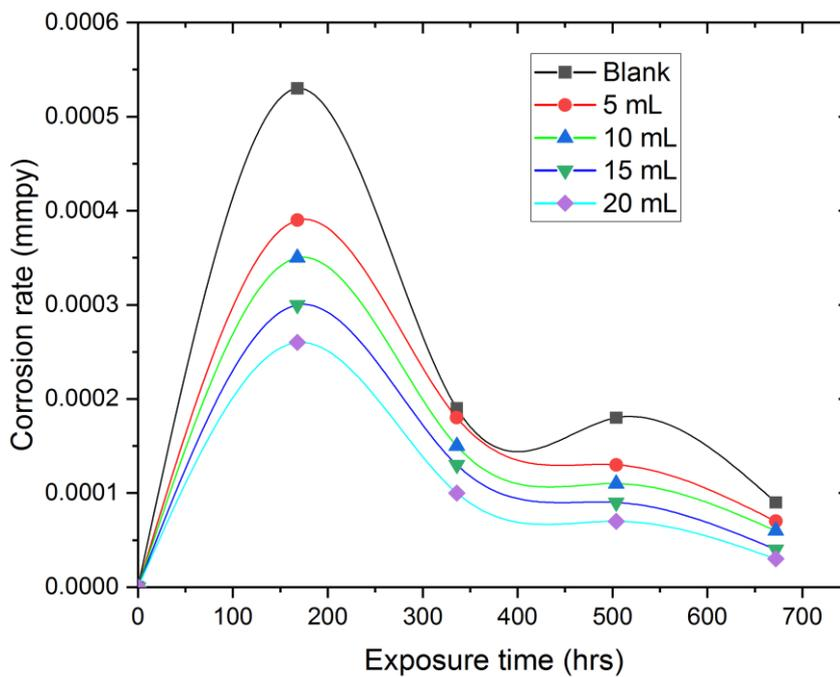
Fig 3: The corrosion penetration rate against exposure time for *Cnidoscopus aconitifolius* in 0.5 M NaCl solution
