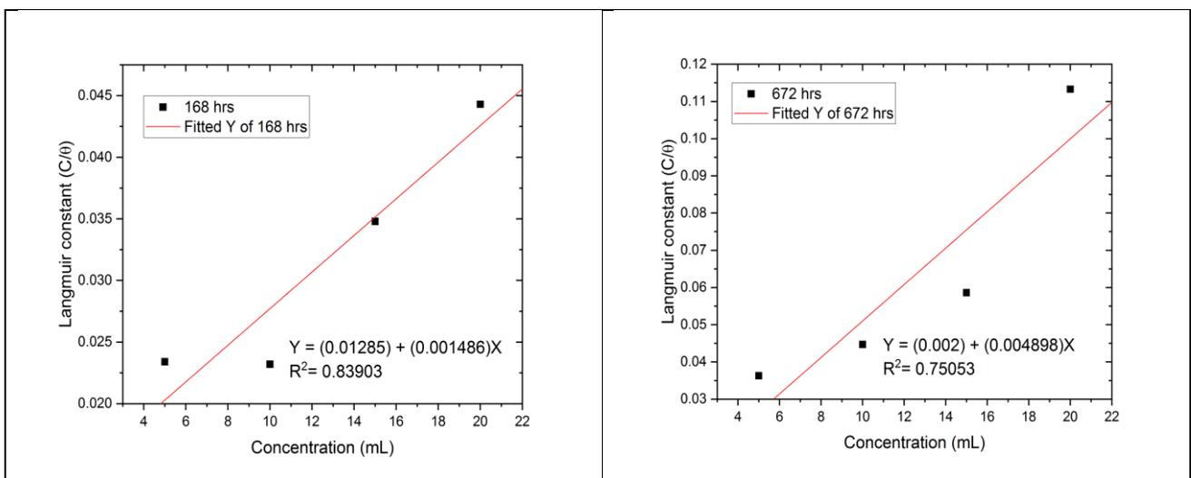
Fig 10: The Langmuir adsorption isotherms for *Cnidoscopus aconitifolius* in 1.0 M H<sub>2</sub>SO<sub>4</sub> at 168 and 672 hours exposure times
