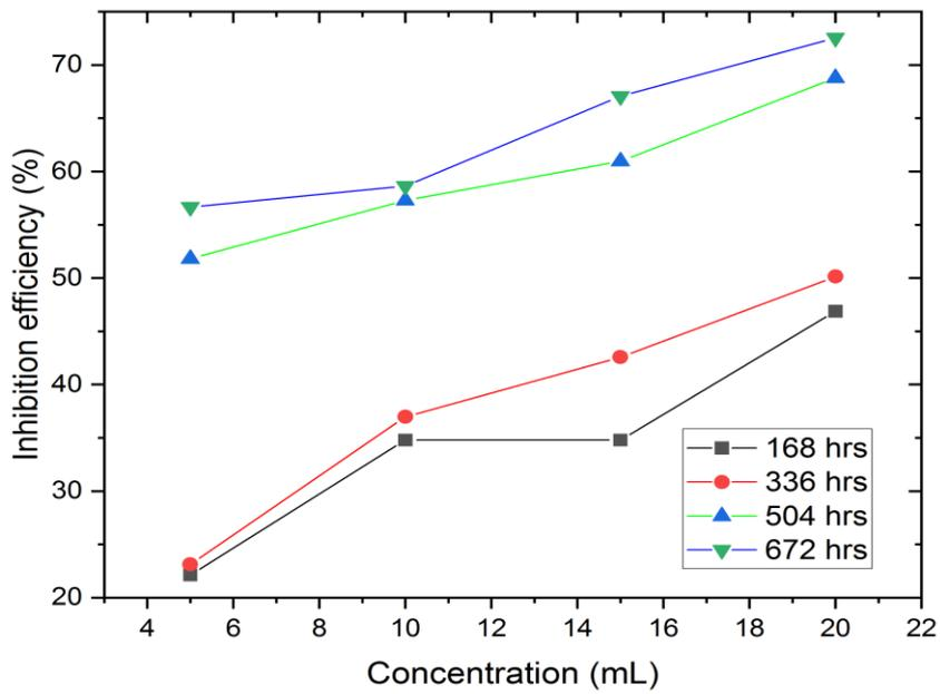
**Fig 6: Inhibition efficiency against extract concentration for *Cnidoscopus aconitifolius* in 1.0 M H<sub>2</sub>SO<sub>4</sub>**
