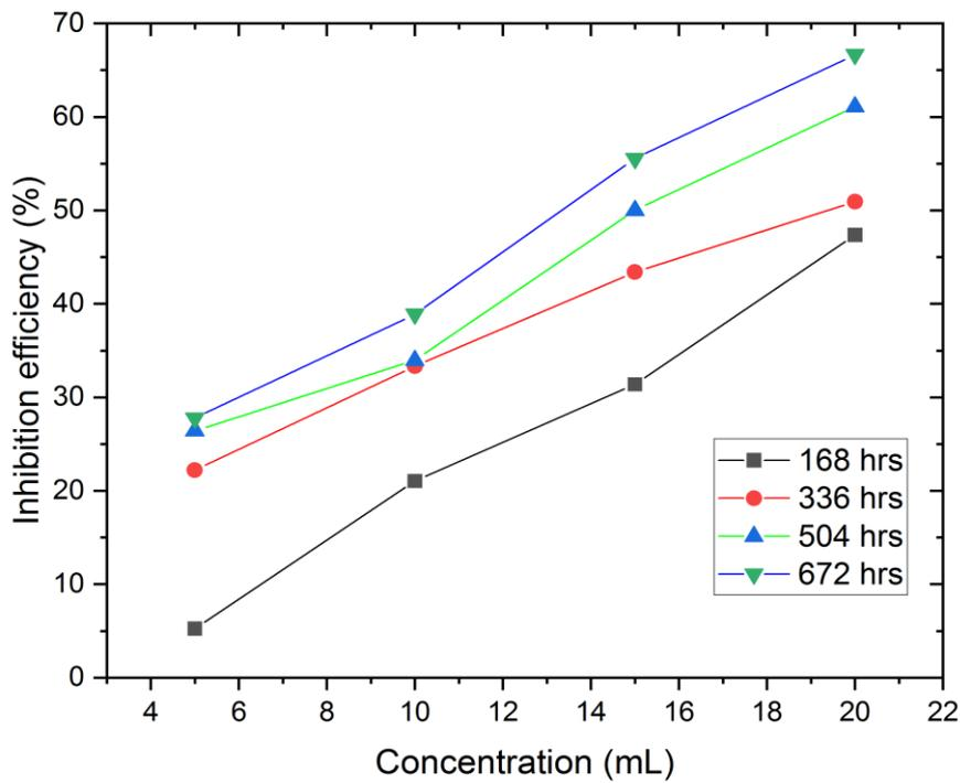
**Fig 7: Inhibition efficiency against extract concentration for *Cnidoscopus aconitifolius* in 0.5 M NaCl solution**
