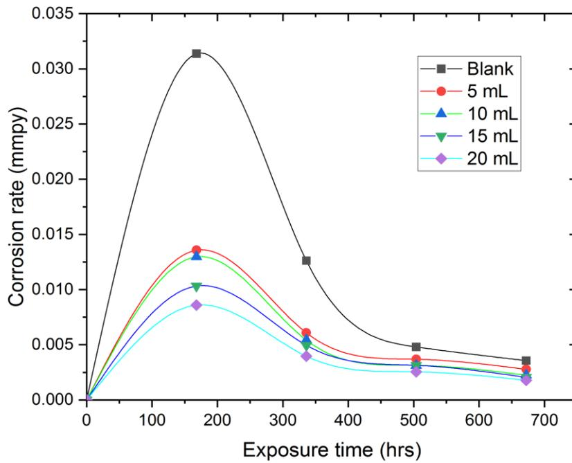
Fig 2: The corrosion penetration rate against exposure time for *Cnidoscopus aconitifolius* in 1.0 M H<sub>2</sub>SO<sub>4</sub>
