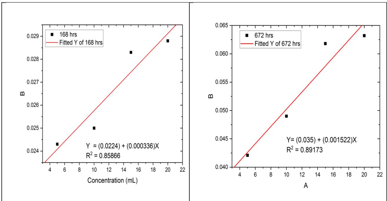
**Fig 12: The Langmuir adsorption isotherms for *Cnidoscopus aconitifolius* in 1.0 M NaCl solution at 168 and 672 hours exposure times**
