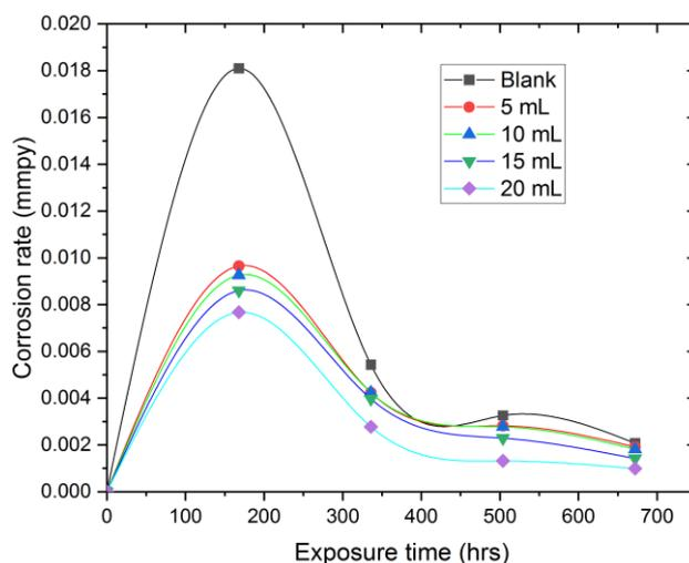
**Fig 1: The corrosion penetration rate against exposure time for *Cnidocolus aconitifolius* in 0.5 M H<sub>2</sub>SO<sub>4</sub>**
