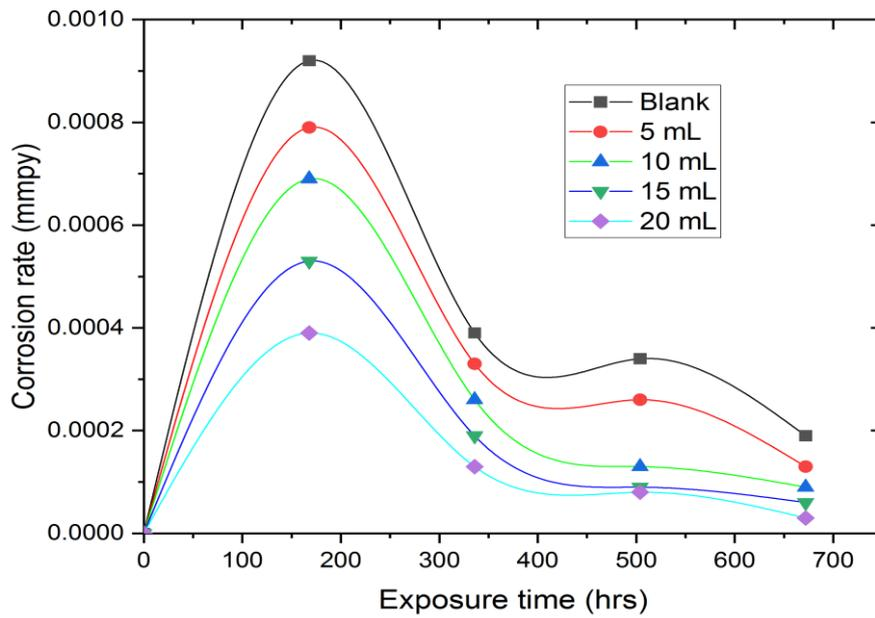
Fig 4: The corrosion penetration rate against exposure time for *Cnidoscolus aconitifolius* in 1.0 M NaCl solution
