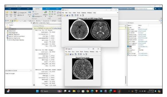
Upon comparison, the fused images generated from both platforms—Xilinx ISE and MATLAB—were found to be consistent in terms of pixel values and overall image quality. This cross-verification confirms the accuracy of the Verilog code and demonstrates the successful hardware realization of the DWT-based image fusion process. Furthermore, it validates that the
