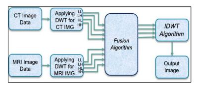
The fusion methodology involves acquiring CT and MRI images in 8x8 grayscale, followed by DWT using Haar wavelets. DWT decomposes images into frequency components, which are fused using averaging rules. The Inverse DWT (IDWT) reconstructs the final fused image. Verilog modules are developed to perform DWT, fusion, and IDWT. Simulation and synthesis are conducted using Xilinx ISE, while MATLAB serves for verification.
