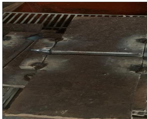
Fig. 1: Joint fit-up of Sample AISI 1018 steel
