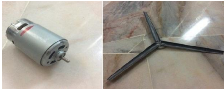
Fig 10: The 12V DC motor and blade made from PVC
