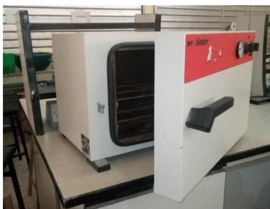
Plate 2: Electric Oven Dryer
