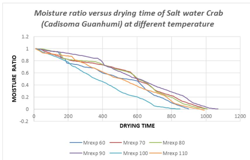
Fig 1: Moisture ratio versus drying time of Salt Water Crab (*Cadisoma Guanhumu*) at different temperature
