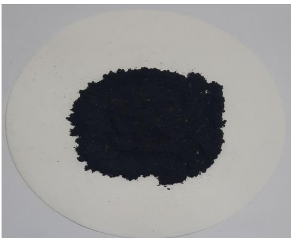
Fig 3: Activated carbon from charcoal with H_3PO_4
