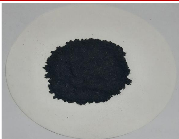
Fig 2: Activated carbon from charcoal with H_2SO_4
