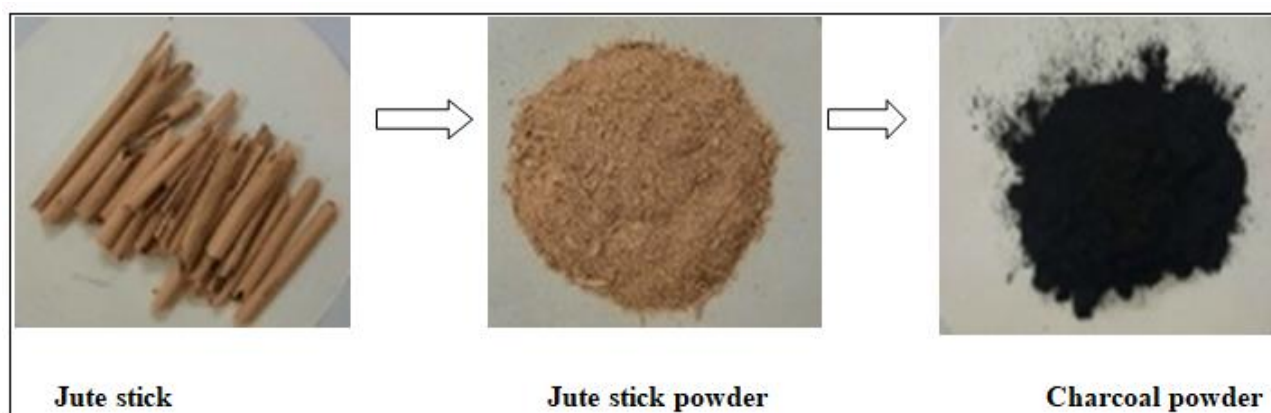
Fig 1: Preparation of activated carbon from jute stick charcoal
