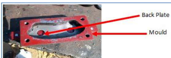
Plate-6b: Mould of Toyota Camry 1998
