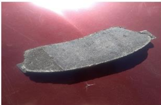
Plate-5: Toyota Camry 1998 Brake pad
