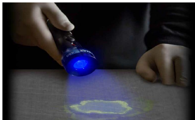
Figure 11: UV light makes the stain visible [12]
