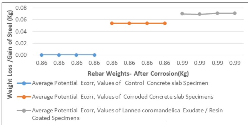
Figure 3.7A: Average Rebar Weights- After Corrosion (Kg) versus Weight Loss /Gain of Steel (Kg)
