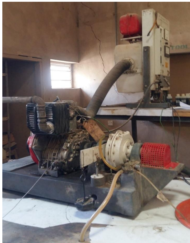
Plate-VI: Complete diesel engine test bed
