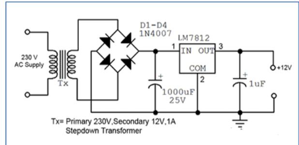
**Fig-3: Power Supply Circuit**
