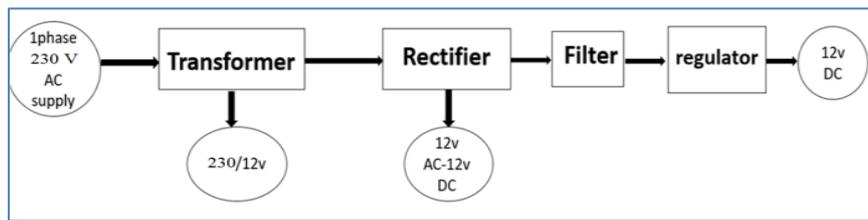
Fig-1: Power supply block diagram
