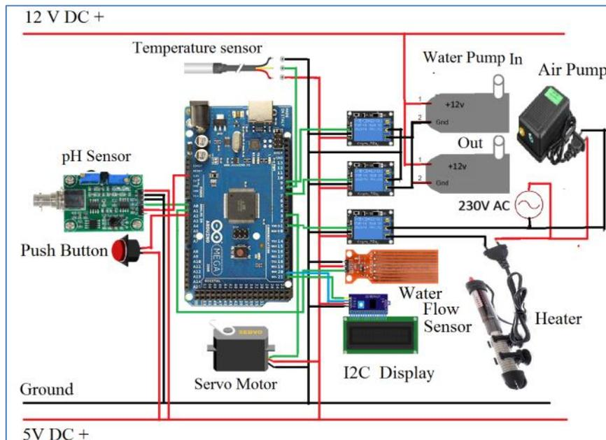
**Fig-4: Main Circuit Diagram of Aqua monitoring system**
