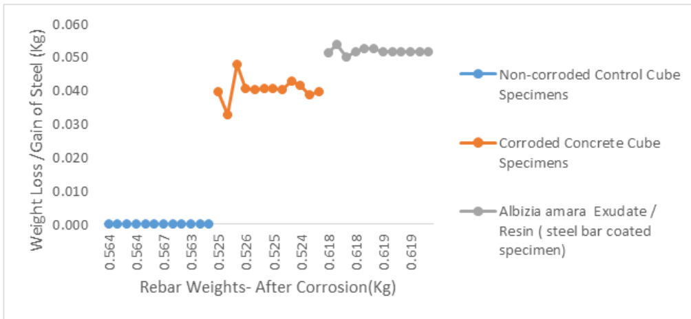
Figure 6: Rebar Weights- After Corrosion versus Weight Loss /Gain of Steel
