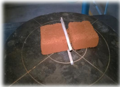
Fig-13: Splitting of a brick after applying of a load
