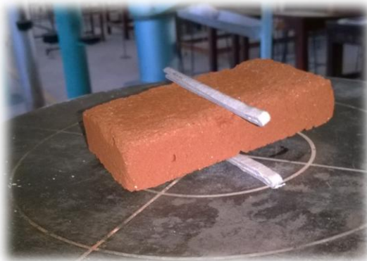
Fig-13: Splitting of a brick after applying of a load
