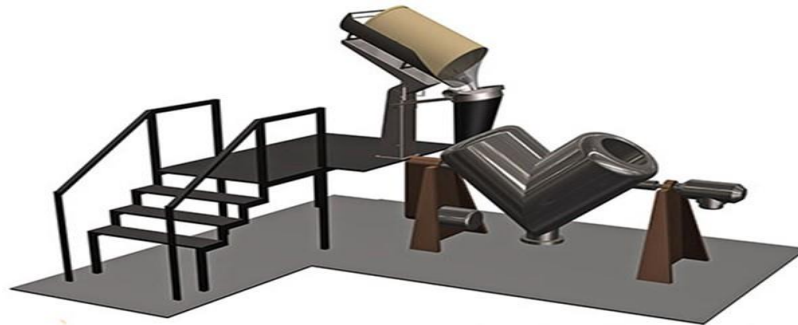
Fig-5: A view of a V-blender [17]
