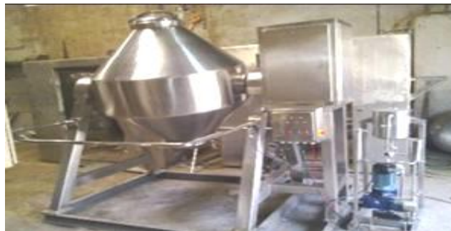
Fig-6: A double cone mixer [21]
