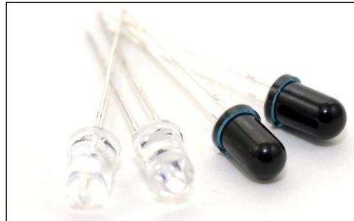
Fig-6: Infrared LED (Sensor)
