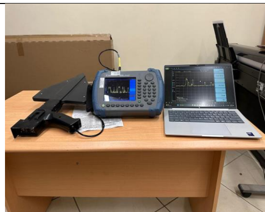
Figure 4: Showing the Spectrum Analyser measurement set-up
