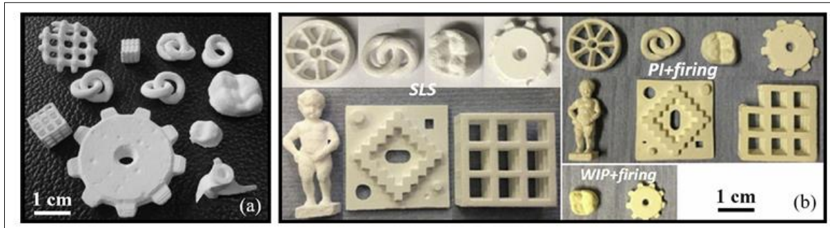
Fig. 19: Complex ceramic parts produced by SLS: (a) \text{Al}_2\text{O}_3 parts with the assistance of quasi-isostatic pressing and final firing [73]; (b) 3YSZ parts after SLS and after combination with pressure infiltration (PI)/warm isostatic pressing (WIP) and final firing [74].
