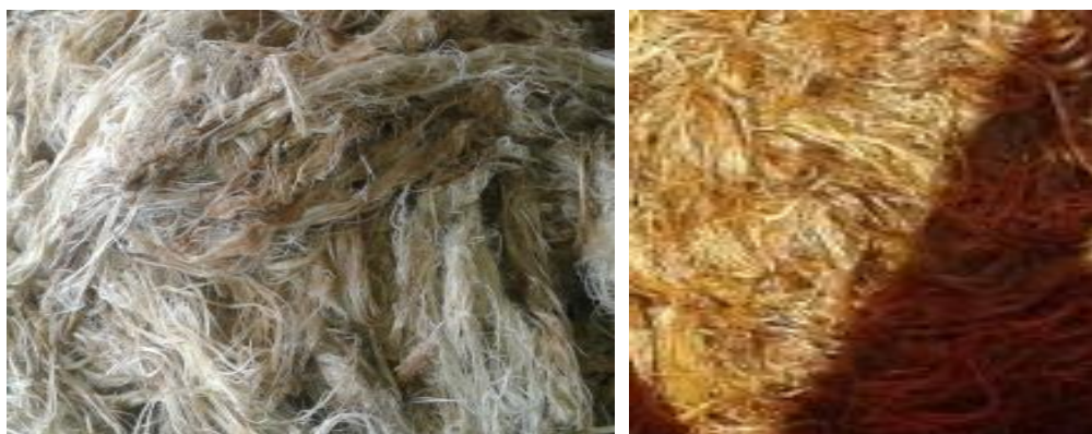
Fig 2: Dried fibre of plantain pseudo-stem
