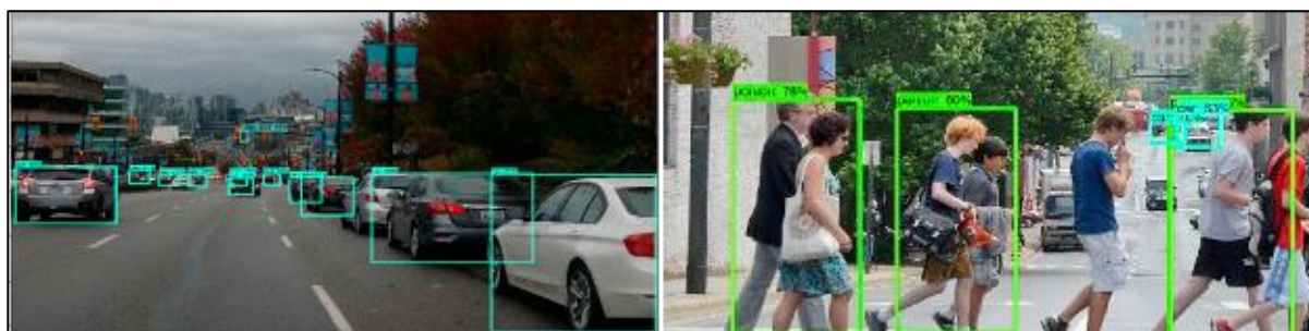
Fig-2: Detecting cars and persons in images applying Deep learning and Faster-RCNN-Inception-V2 model
