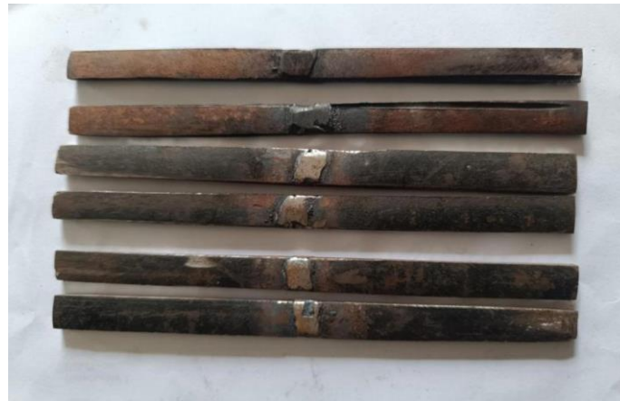
Fig. 1: Samples of UNS G10350 carbon steel pipe weld for tensile testing
