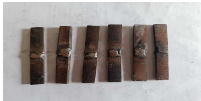
Fig. 2: Samples of UNS G10350 carbon steel pipe weld for hardness testing
