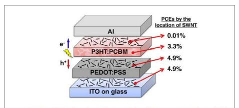
Figure 2. Illustration of a work reported in reference 6. SWNTs located either above or below the hole-transporting layer of OSCs perform the best (the numbers indicate PCEs obtained with different position of the SWNT layer).
