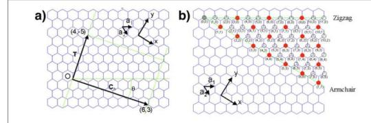
**Figure 1.** a) Definition of chiral vectors in a hexagonal lattice. b) For a SWNT chirality of (n,m), if the value of (n-m)/3 is an integer, the SWNT is metallic. The red dots represent metallic SWNTs.
