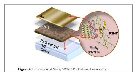
This optimal hybrid structure, devoid of an adhesive layer, exhibited a synergistic effect that facilitated effective separation of electrons and holes. Efficiency scores ranged from 4.7% to 6.11% (Table 1: Report M) when utilizing indene-C60 bisadduct (ICBA)
