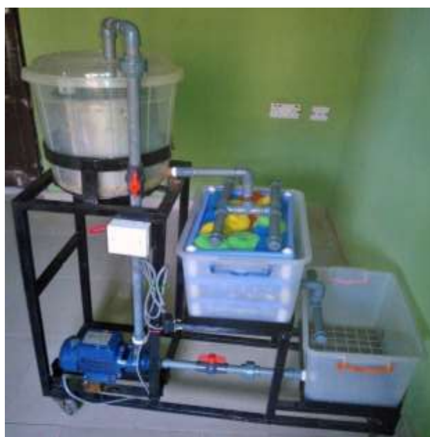
Fig-2: Aerial view of a Fabricated Lab-scale Recirculation Aquaculture Plant
