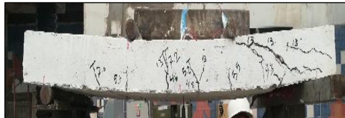
Figure 16: Crack patterns on the surface side of the slab (S30)
