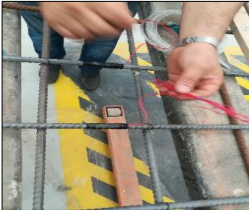
Figure 7: Attaching the strain gauges to the GFRP and Steel bars
