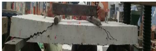
Figure 21: Crack patterns on the other surface side of the slab (F30)
