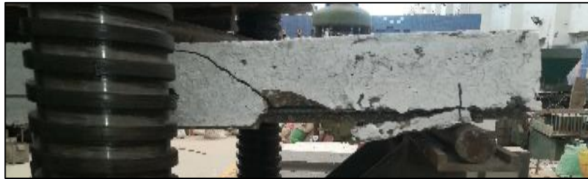
Figure 19: Crack patterns on the other surface side of the slab (S70)
