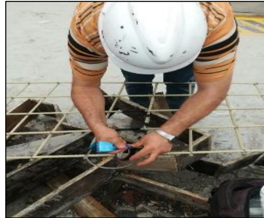
Figure 8: Strain gauges attached on the top concrete surfaces
