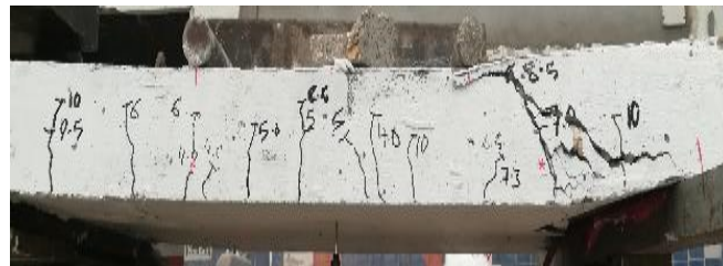
Figure 20: Crack patterns on the surface side of the slab (F30)
