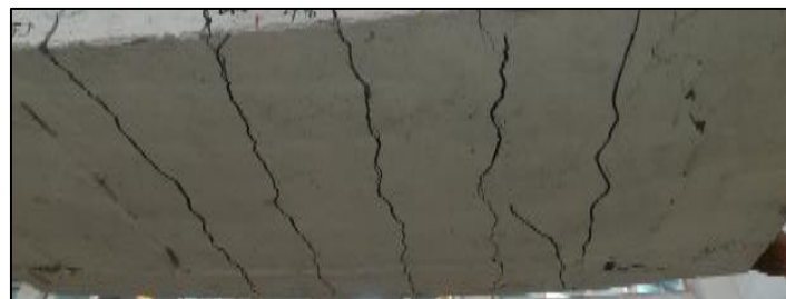
Figure 17: Crack patterns on the bottom surface of the slab (S30)
