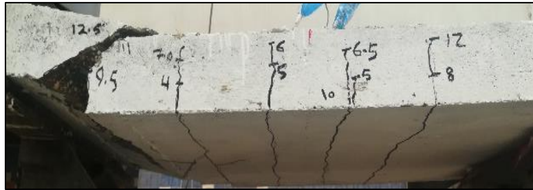
Figure 22: Crack patterns on the surface and bottom side of the slab (F70)
