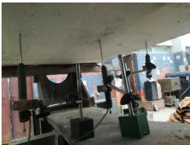
Figure 14: LVDTs location to measure deflection and crack width during the test
