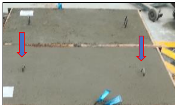
Figure 6: Two lifting anchors bars
