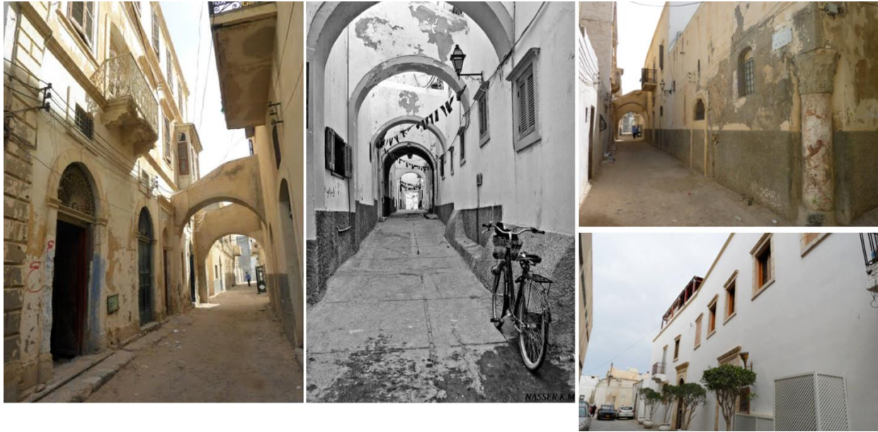
Figure 7: The Hosh is a type of traditional Libyan house, characterized by its linear design with a longitudinal extension parallel to the street, and surrounded on the sides by neighboring houses that vary in height. The structural elements with repeated arches cast shadows on the walls of houses and alleys, which contributes to softening the atmosphere and reducing the effect of direct sunlight. In addition, these shoulders act as architectural supports that enhance the stability of the walls and support their structural structure
