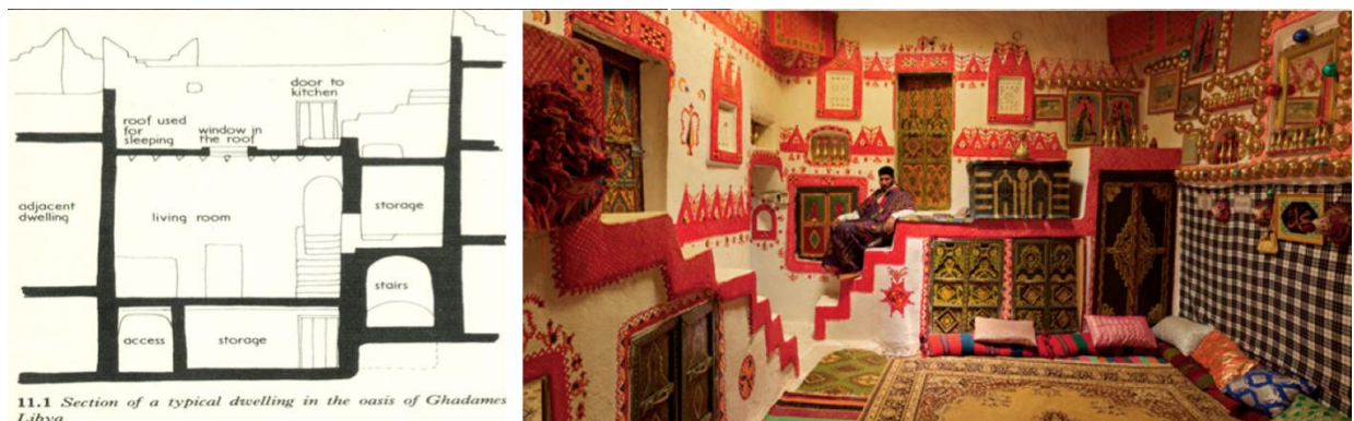
Figure 14: He explains that a tight cluster of houses in Ghadames city creates its own natural cooling system, with the streets protected from direct sunlight by the vertical and compact massing of buildings. This massing helps keep the temperature inside the streets and houses at relatively moderate levels, even on the hottest summer days, providing a comfortable environment for residents without the need for artificial air conditioning systems
