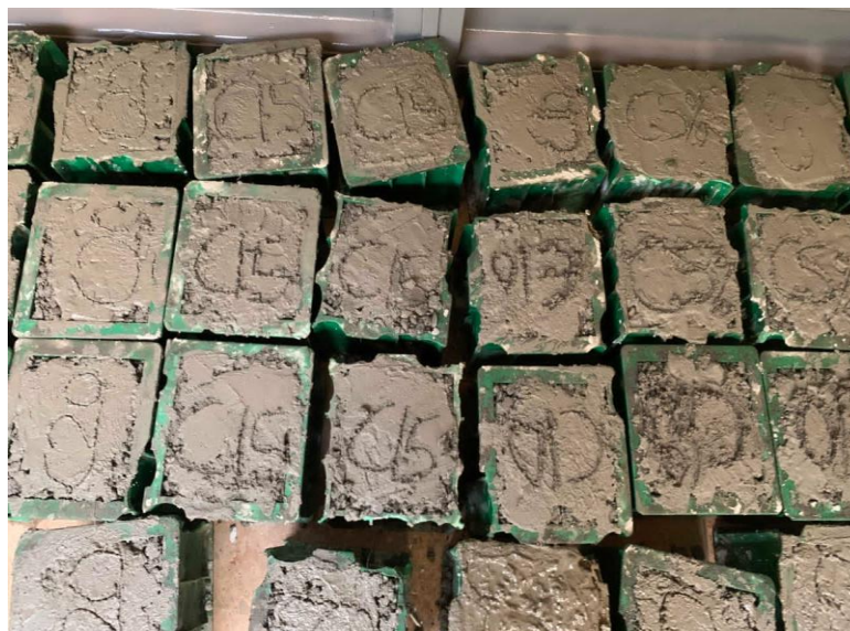
Figure 2: Cast cubes of crushed cow bones
