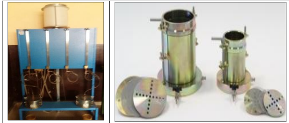
Fig. 4: Equipment for ksat testing using PPR and moulds for compacting the material NF X 30-441, [18]
