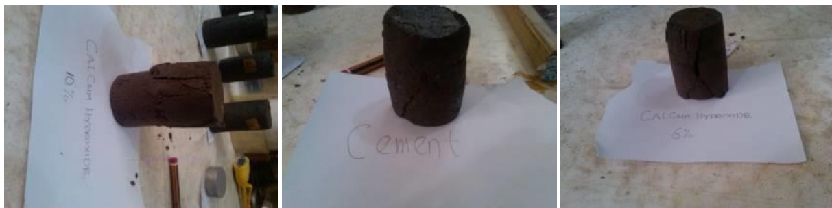
Fig. 4.11: Some Improved Soil samples after UCS test
