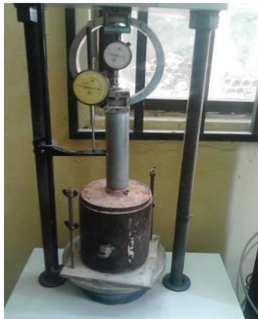
Fig. 4.9: CBR machine set up for CBR test
