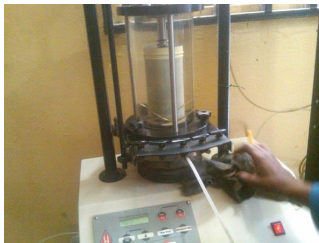
Fig. 4.10: UCS test set up and ongoing experiment
