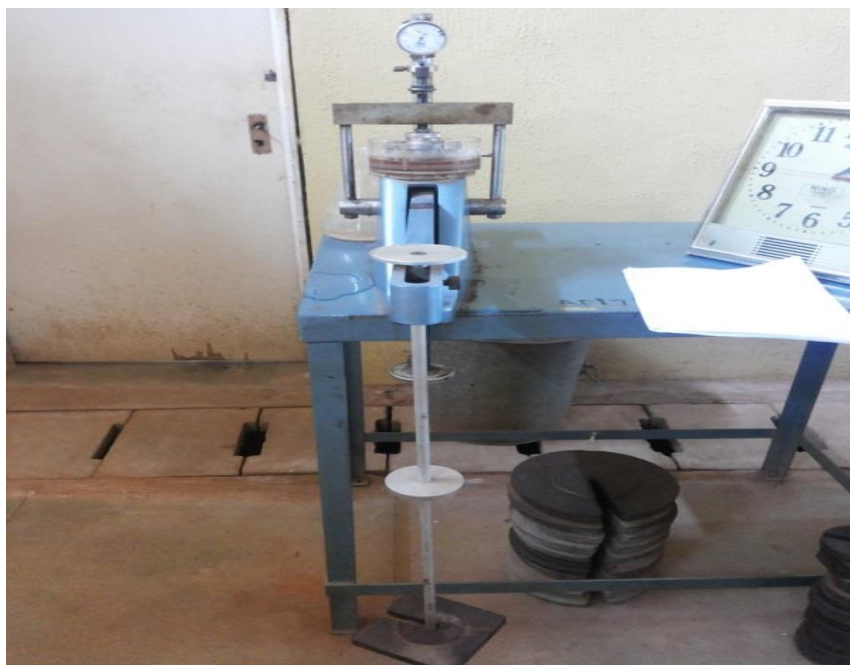
Figure 2.1: Set-Up of Oedometer Apparatus
