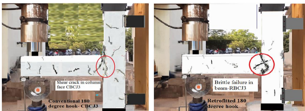
Fig 23. Crack pattern in 180 degree hook .Conventional & Retrofitted anchorage
