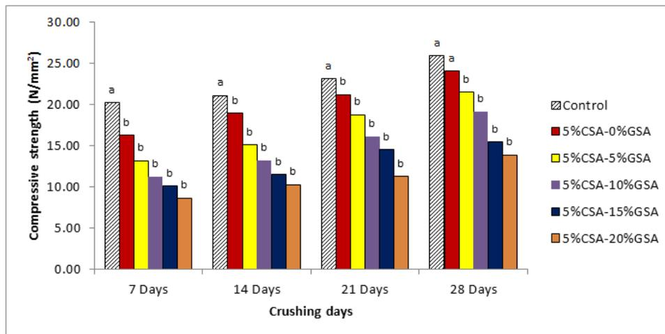
Figure 4: Compressive Strength of CSA-GSA Concrete
