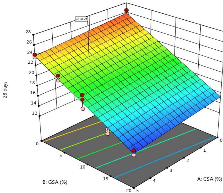
**Figure 5: Optimized 28 Days CSA-GSA Concrete Compressive Strength**
