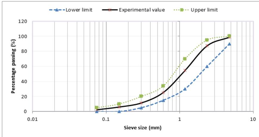
**Figure 1: Particle Size Analysis of Fine aggregate**
