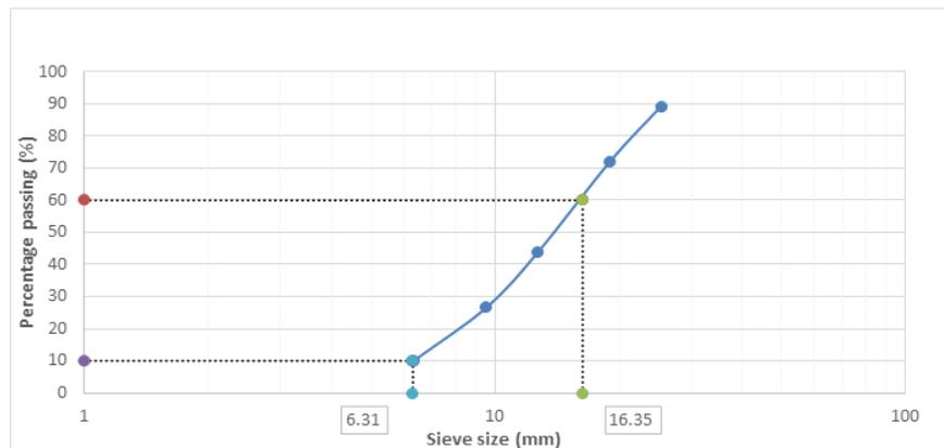
**Figure 2: Sieve Analysis of Coarse Aggregate**
