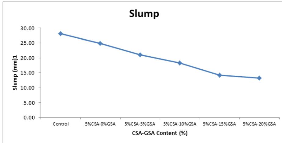
Figure 3: Workability of CSA-GSA Concrete
