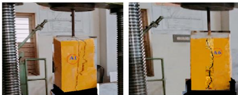
FIG.6B EXPERIMENTAL OBSERVATION OF STRAIGHT ANCHORAGE
