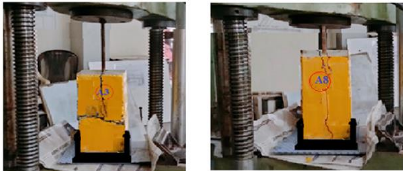
FIG.8B EXPERIMENTAL OBSERVATION OF 180 DEGREE HOOK
