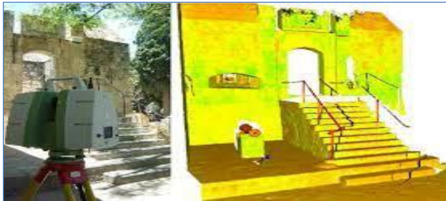
Fig-21: The textured point cloud model with laser and images.
