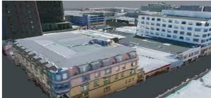
Fig-24: 3D city model by matching aerial laser and terrestrial laser.
