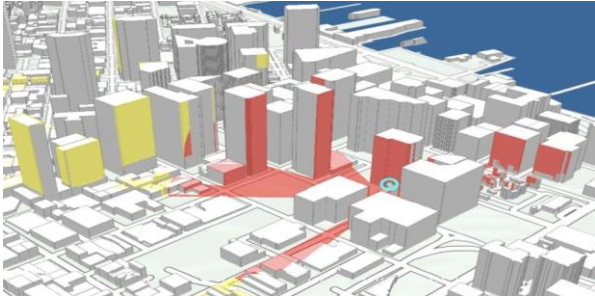
Fig-4: The estimation of the line of sight between every two points from 3D city models [40].
