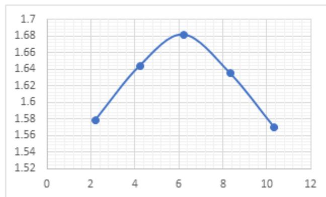
**Fig-6: Compaction result for subgrade soil**
