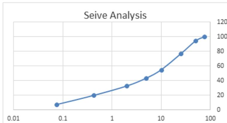
**Fig-5: Sieve analysis for subgrade soil**
