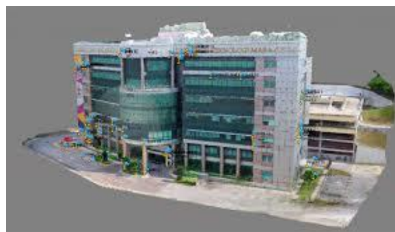
Fig-1: 3D model with the textural data from 3D documentation project using CRP [1].
