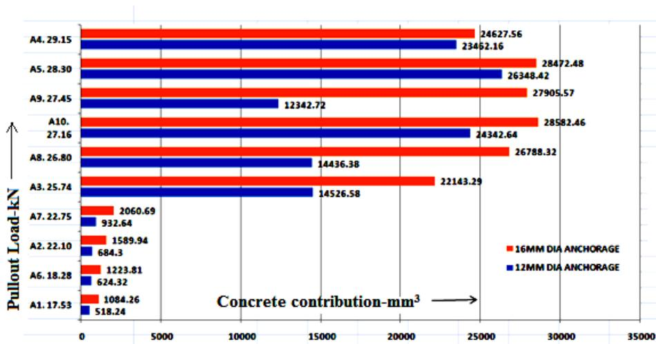
Fig.14 CONTRIBUTION OF CONCRETE IN 12MM & 16MM DIA ANCHORED BAR. IMPACT TEST
