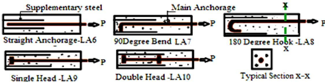
**Fig.6b Retrofitted Anchorage system**
