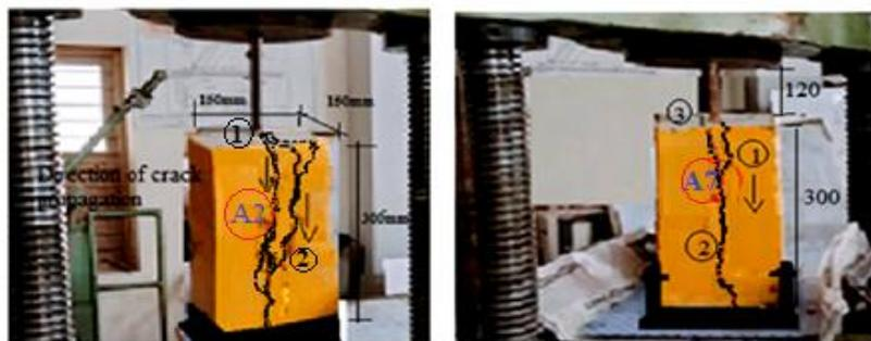
Fig.9a Conventional 90 degree Bend A2 Fig.9b Retrofitted 90 degree Bend A7
