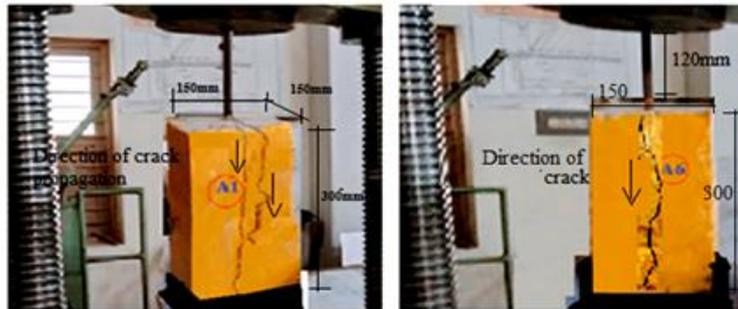
Fig. 8a Conventional Straight Anchorage A1 Fig. 8b Retrofitted Straight Anchorage A6
