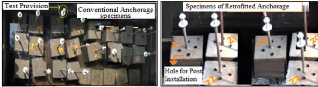
Fig.7a. Test specimens of Conventional Anchorage Fig.7b. Test specimens of Retrofitted Anchorage
