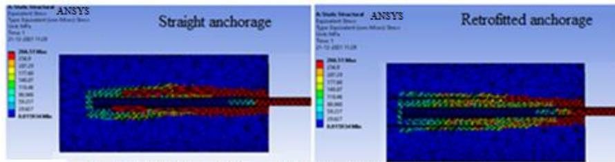
Fig.1 ANSYS modelling of Straight & Retrofitted anchorage
