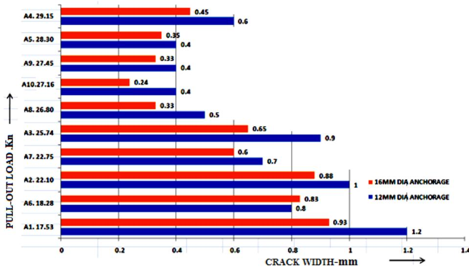
Fig.15 CRACK WIDTH OF 12mm & 16mm SIZE ANCHORED BAR-IMPACT LOAD
