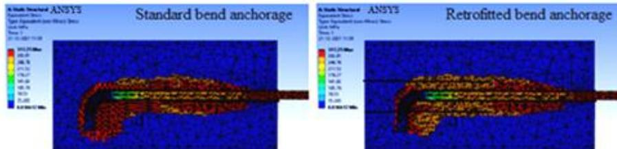
Fig.2 ANSYS modelling of normal stress in 90 degree Bend & Retrofitted anchorage
