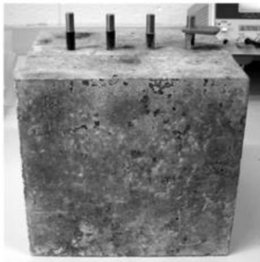
Figure 4: Concrete cube with embedded electrodes (McCarter et al. , 2009)
