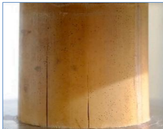
Fig-9: The splitting failure mode of a bamboo specimen after the compression strength test
