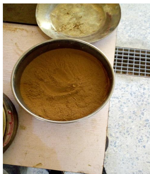
Fig-1: Clay Sample Passing 40 Micron BS Sieve
