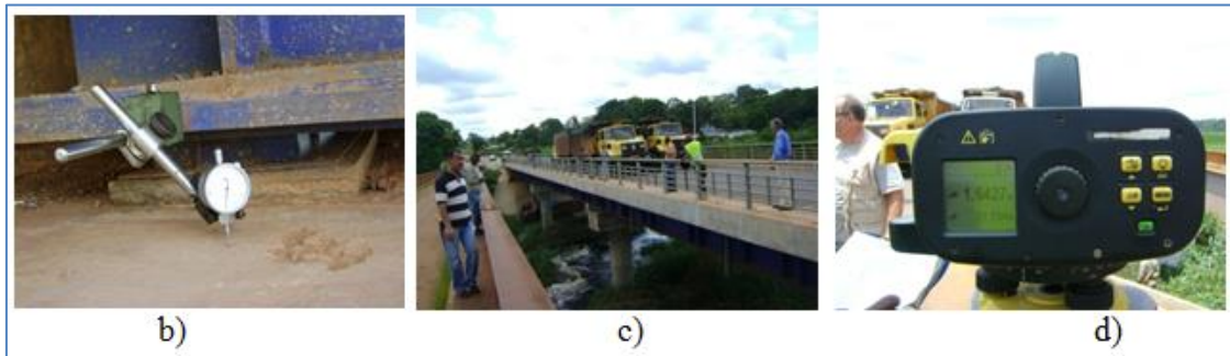
Fig-5: Experimental Setting: Trucks a) convoy position; b) comparator position; c) static test loading; and d) the topographic deflectometer
