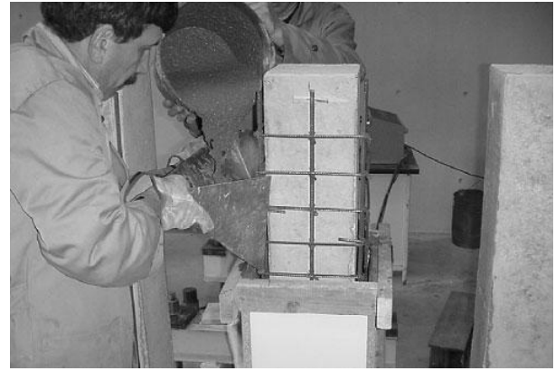
Fig-4: Casting concrete jacket
